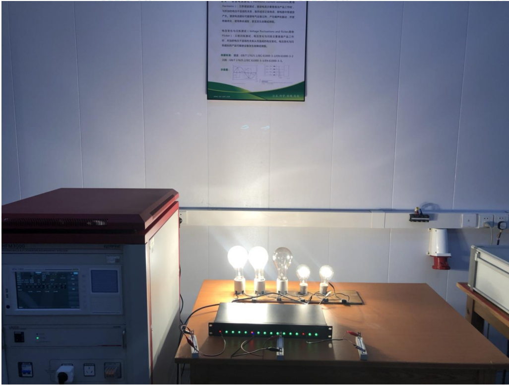
Test Setup Photo of Harmonic & Flicker Measurement
