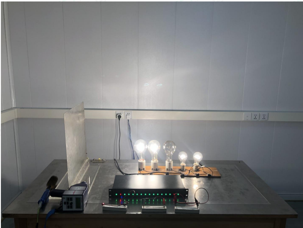
Test Setup Photo of Electrostatic Discharge Test
