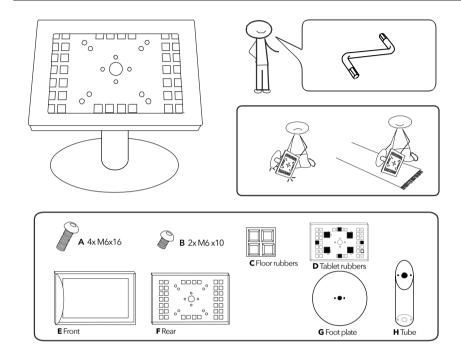
**Before you start:** Determine and fix cell rubbers [**D**] position with tablet in the exact middle of the casing. (See manual - *Fixing the rubbers*) Also determine the postition of the screen; Portrait or landscape.
