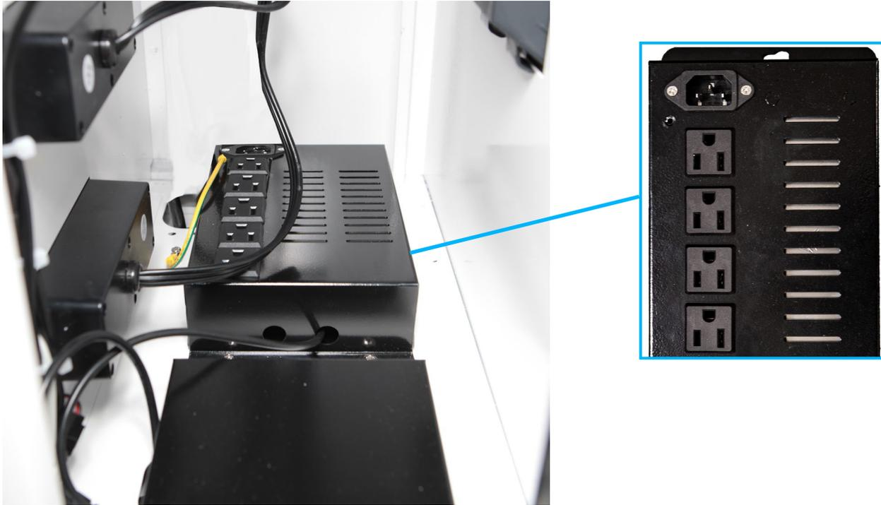
**Step-7:** One at a time, feed the Power Input Plug, then the Power Strip Plug through the pass-through hole located near the back.
