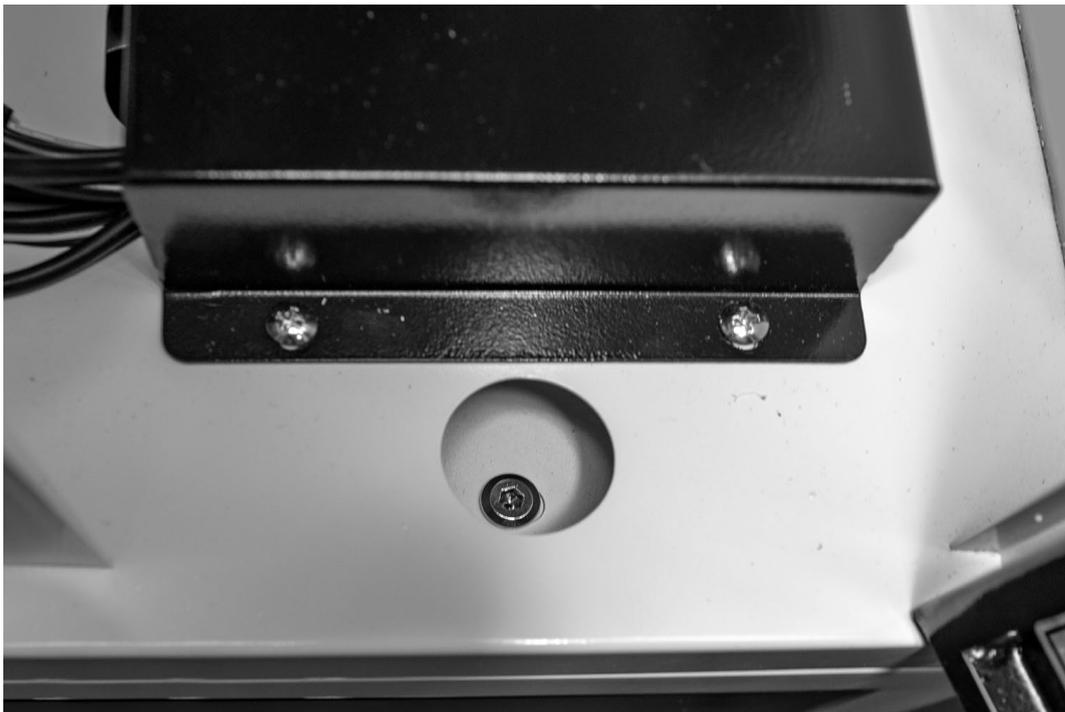
**Step-12:** Working in the back, use the Hex wrench to remove the (4) Hex bolts from the middle left and middle right edges.
