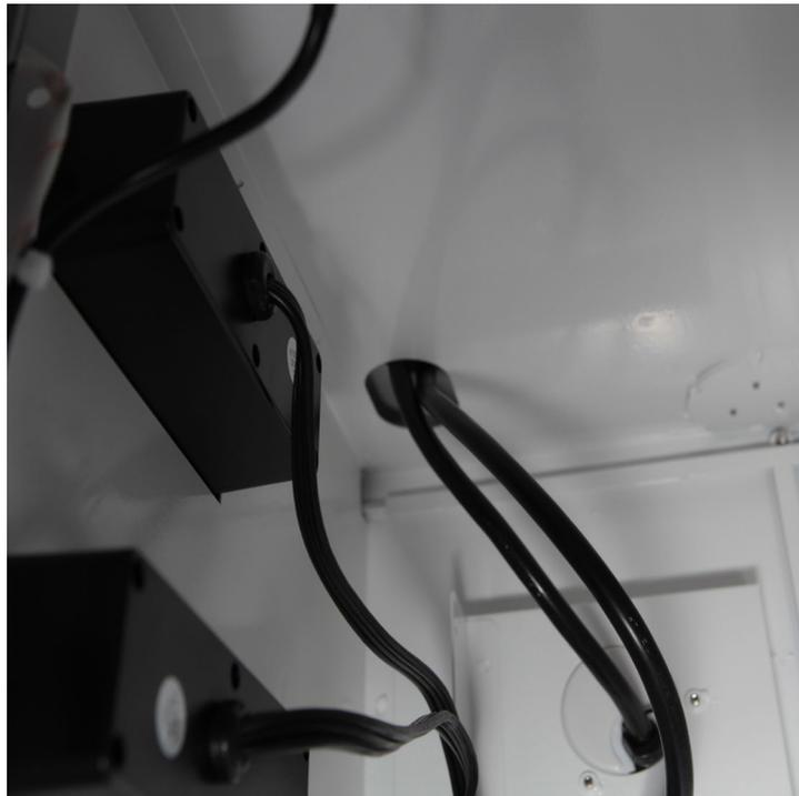
**Step-8:** Plug both the Power Input Plug AND Power Strip Plug into the Power Supply.
