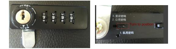
2.2.2Turn the switch to the close, then confused the code, the lock will be closed. When want to open turn the new code 9999.
