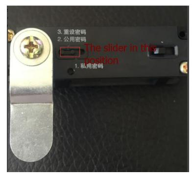
2.2.1 Set the new code example "9999", then turn the slider to the position 1.
