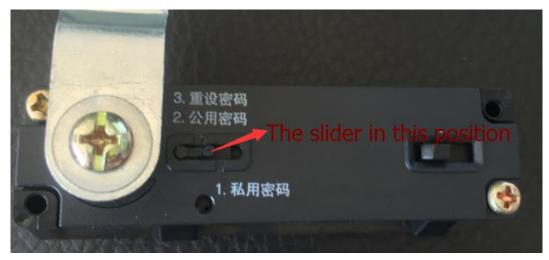
Example, reset the code "9999" then turn the switch to the close statue and Sliding the slider to the right (the position 1)
