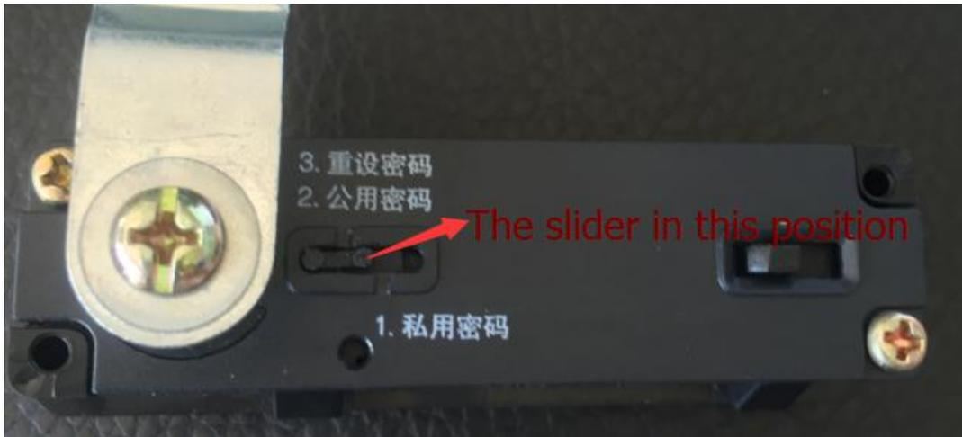
Example, reset the code "9999" then turn the switch to the close statue and Sliding the slider to the right (the position 1)
