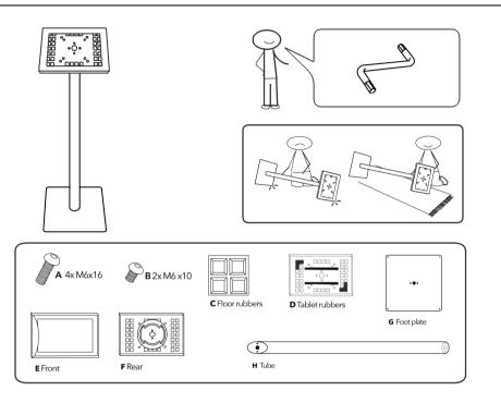
**Before you start:** Determine and fix cell rubbers [**D**] position with tablet in the exact middle of the casing. (See manual - *Fixing the rubbers*)
