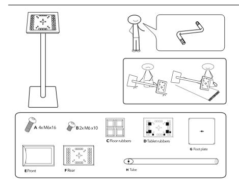
**Before you start:** Determine and fix cell rubbers [**D**] position with tablet in the exact middle of the casing. (See manual - *Fixing the rubbers*)
