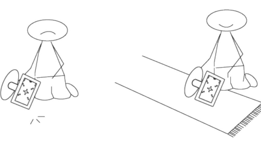
NOTE: Use a soft underlayment during assembly to avoid damage
