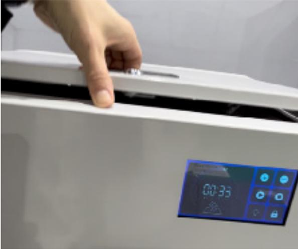
Access CNC charging hub by unlocking top panel, lift panel using provided handle.
