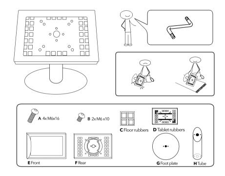
**Before you start:** Determine and fix cell rubbers [**D**] position with tablet in the exact middle of the casing. (See manual - *Securo Fixing the rubbers*)
